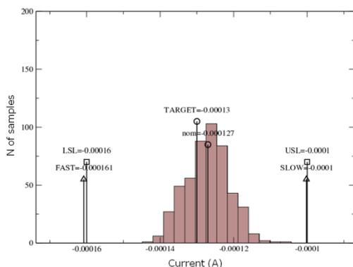
Fig. 2. Saturation current of device A. The y-axis show the number of Monte Carlo iterations (total: 1000). It can be seen that there is a residual difference between the nominal value of the model parameter and the real target value, due to a non-perfect centering.
