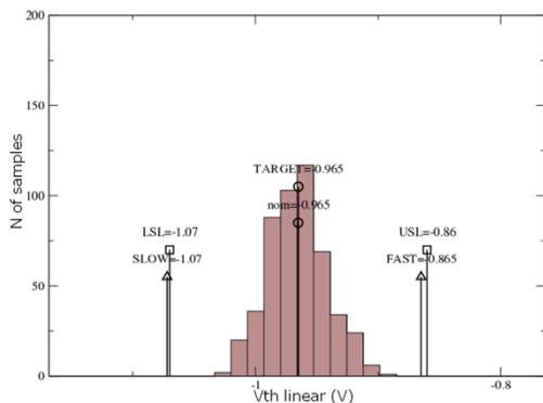
Fig. 3. Threshold voltage in the linear regime of device A. The y-axis show the number of Monte Carlo iterations (total: 1000).
