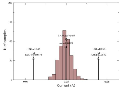
Fig. 1. Saturation current of an n-MOSFET device. The target value is the desired nominal current, while the “nom” value is the actual current reproduced by the model. USL and LSL are the maximum and minimum allowed currents, whereas FAST and SLOW are the currents we would like to get with a corner simulation. A Monte-Carlo simulation is also shown for comparison (total number of samples: 1000).
